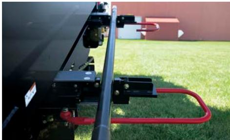
**VARIETY OF ROD OPTIONS.** The D40x55 S3 is available with a range of drill rod options, including a 10' (3 m) length in 2.38" (6 cm) or a 2.63" (6.7 cm) diameter, and a 15' (4.6 m) length in a 2.63" (6.7 cm) diameter. A variety of rod options allows the drill to be configured to the specific needs of the contractor.
