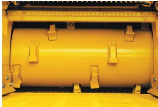
**The one, the only, Duplex Drum.** The patented Duplex Drum cutting system offers optimum cutting performance with full surface coverage of the material. In addition, it offers the latest technology in hammer design and replacement procedures in the industry. Maintenance time is reduced due to easy hammer and cutter block change out. Plus, hammers and cutter blocks are reversible, therefore nearly doubling hammer life.
