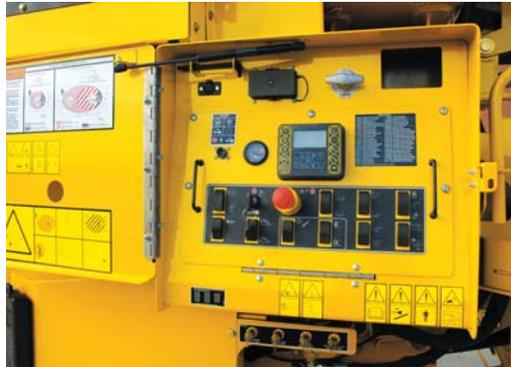
**Control panel.** A centralized control station provides real time performance information and full instrumentation. The control panel is also equipped with diagnostic ports for monitoring systems and troubleshooting.
