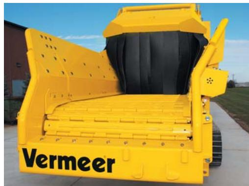
**Formed alloy slat and chain feed table.** The HG4000TX feed table features a solid floor design with continuous support of the infeed chain to help improve structural support and increase chain life.
