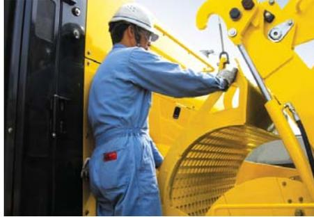
**Easy access screens are engineered with top-loading design** to allow the operator to change screens more easily, and in less time than conventional side loading screens. A variety of screen sizes are available to meet specific project needs.
