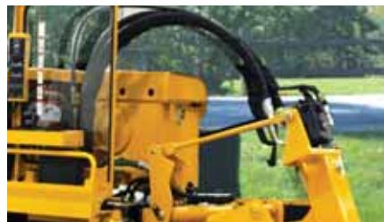
**Direct drive hydrostatic pump and gearbox** eliminates clutch and belt-drive maintenance. Cutter wheel stopping time is reduced with no-maintenance hydrostatic braking.
