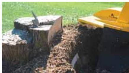
**High cutter wheel** moves away from the machine as the boom drops, increasing the maximum cutting width. The SC852 gives you a cutting height of 31" (79 cm) above ground and 25" (64 cm) below — the deepest cut in its class.
