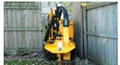
**Front-mounted controls** offer maneuverability in confined spaces by allowing the operator to walk in-line with the machine.
